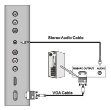
Connect the RGB output of the PC to the VGA in jack on the set Connect the PC AUDIO output of the PC to the PC AUDIO in jack on the set Select the VGA input source with using SOURCE button.
